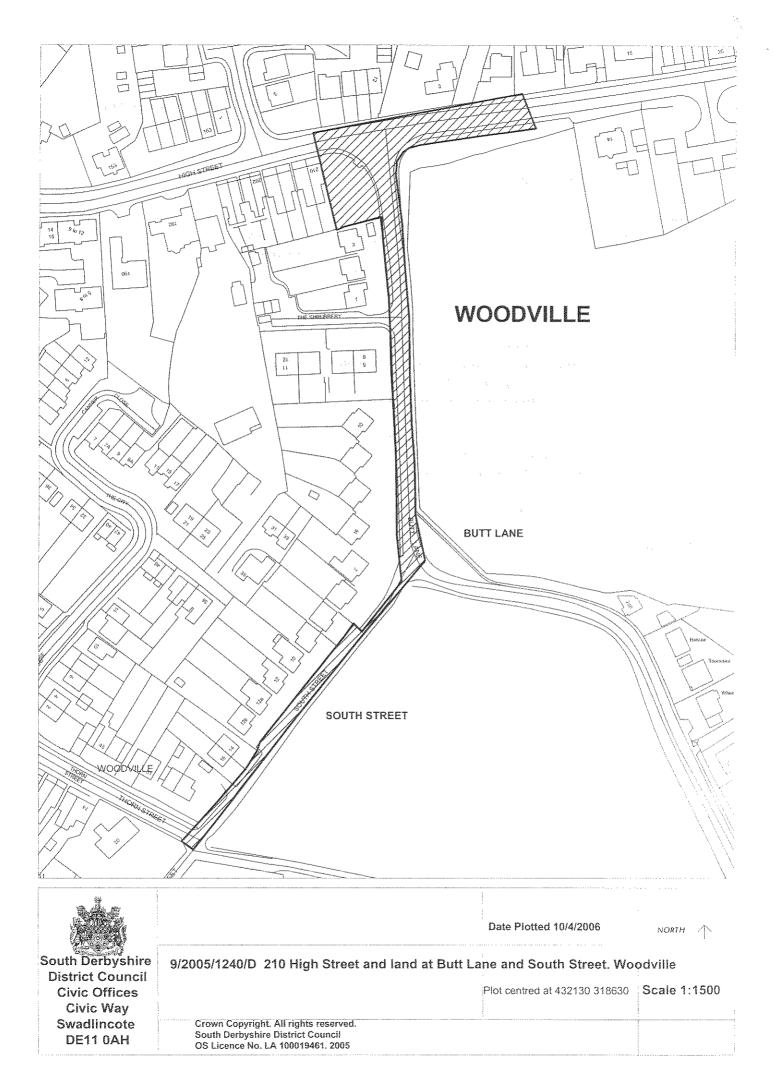
The link road will run parallel to the eastern side of Butt Lane for some 170m and a new junction will be formed with the A511 resulting in the northern end of Butt Lane being terminated as a cul-de-sac. A spur road from the link road would connect to South Street at a point some 15m north east of the junction with Thorn Street. The section of South Street between Butt Lane and Thorn Street would be improved to adoptable standard.
