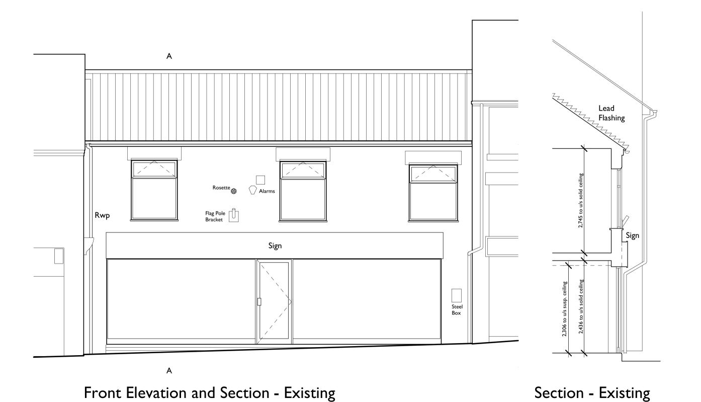
Existing first floor windows to be carefully removed by contractor and replaced with new timber windows as shown and specified.
