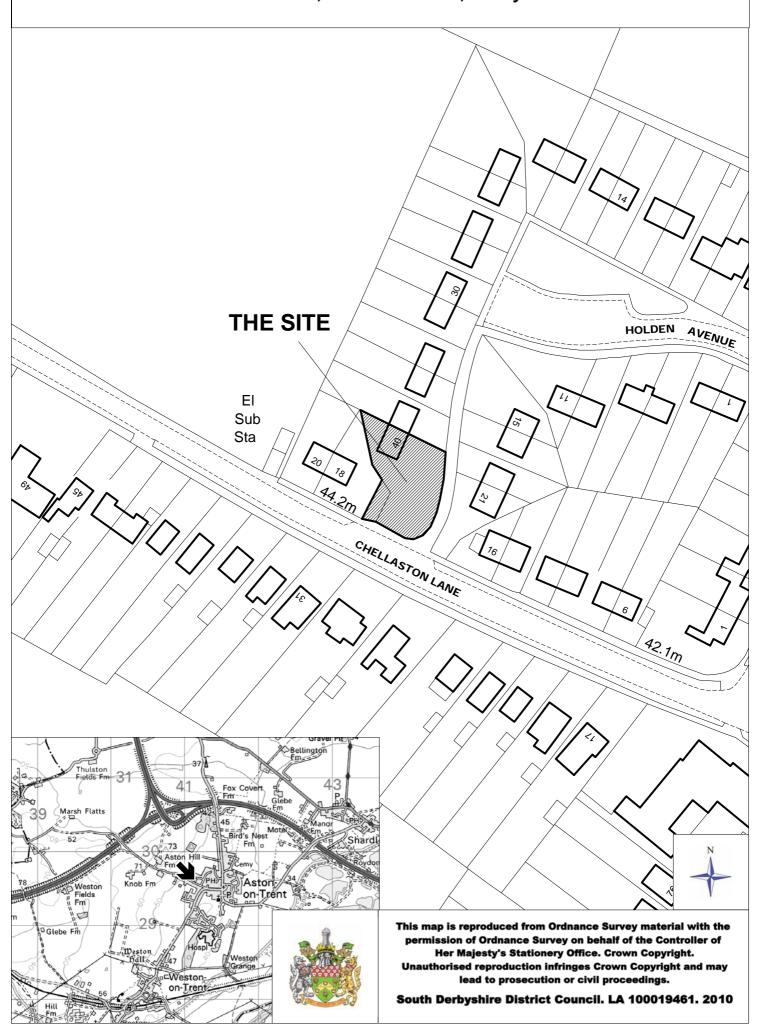
The applicant has submitted supporting details on how access viability at 40 Holden Avenue could be improved. The applicant proposes to remove the existing gateposts, and cut the hedge bordering Chellaston Lane down to 600mm, to give a 2.4m x 43m visibility splay to comply with the County Highway Authority's requirements.
